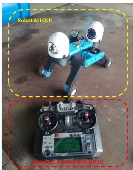
Figure 11. ALLQU robot and Operational Control Unit (OCU)
