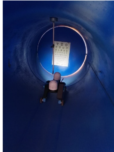
Figure 15. ALLQU robot in the ventilation duct, performing vision tests using a SNELLEN chart.
