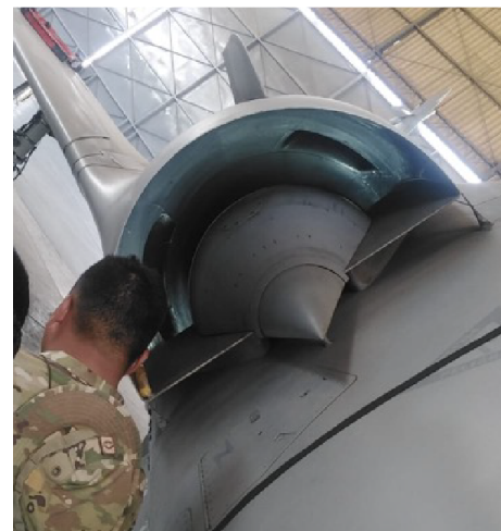
Figure 14. Ventilation duct of the Mirage aircraft
